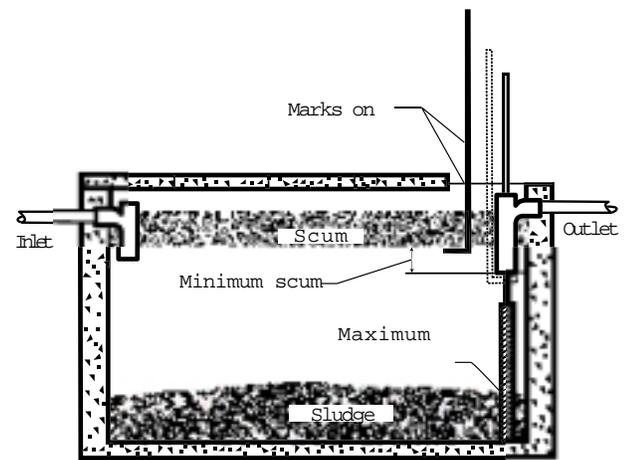
Procedures for measuring the accumulation of sludge and scum layers in a septic tank. Source: *Septic Tank Maintenance*. OSU Extension Facts No. 1657. Delbert Schwab, J. H. Armstrong, S. Harp. Oklahoma State University Extension.
