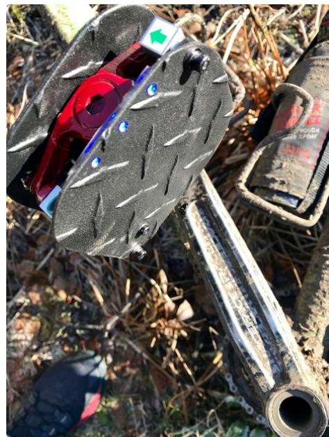
the sensor with each pedal rotation. I used a web based calculator that estimates your power output on a hill climb given your weight, height of your climb and time and found the result was within spitting distance of what the meter was reading.
