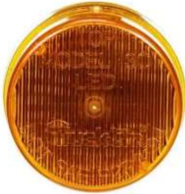
**A: Reflex Reflector- ALL LIGHTS USED AS COMBINATION LIGHTS AND REFLECTORS MUST HAVE AN "A" RATING.**
