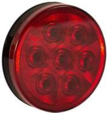
*Example: The light below is a 4" Stop, Turn, Tail 3 wire LED light that is commonly sold for this purpose. This light **DOES** have the proper DOT IST SAE code stamped on the lens and **CAN** be used as a combination Stop, Turn, Taillight, but **DOES NOT** have the "A" code and **CAN NOT** be used as a combination light and reflector, according to federal DOT guidelines.*
