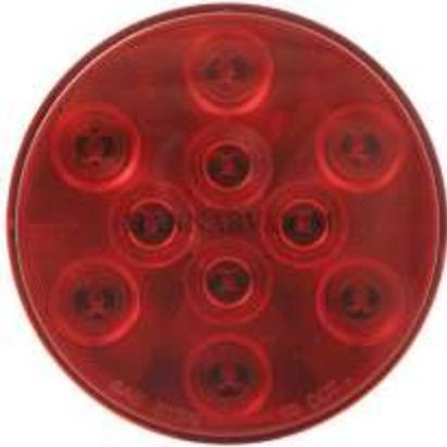
*Example: The light below is a Common Stop, Turn, Tail 3 wire LED with side rear marker light that is commonly sold for this purpose. This light **DOES** have the proper DOT AIST SAE code stamped on the lens and **CAN** be used as a combination Stop, Turn, Taillight, and **DOES** have the "A" code and **CAN** be used as a combination light and reflector, according to federal DOT guidelines.*
