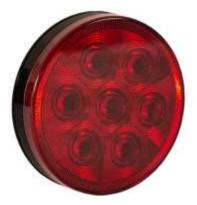
Example: The light below is a 4" Stop, Turn, Tail 3 wire LED light that is commonly sold for this purpose. This light <u>DOES</u> have the proper DOT IST SAE code stamped on the lens and <u>CAN</u> be used as a combination Stop, Turn, Taillight, but <u>DOES NOT</u> have the "A" code and <u>CAN NOT</u> be used as a combination light and reflector, according to federal DOT guidelines.
