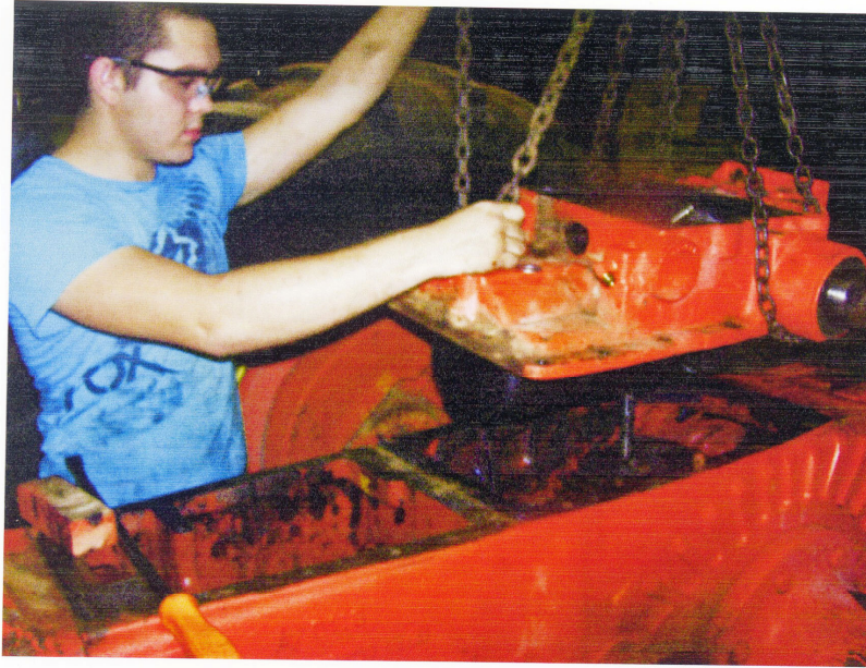
Removing lift assembly
