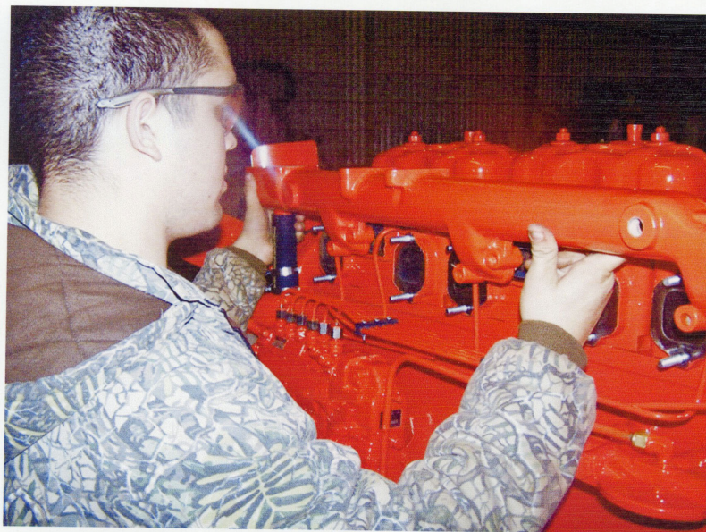
Mounting water manifold
