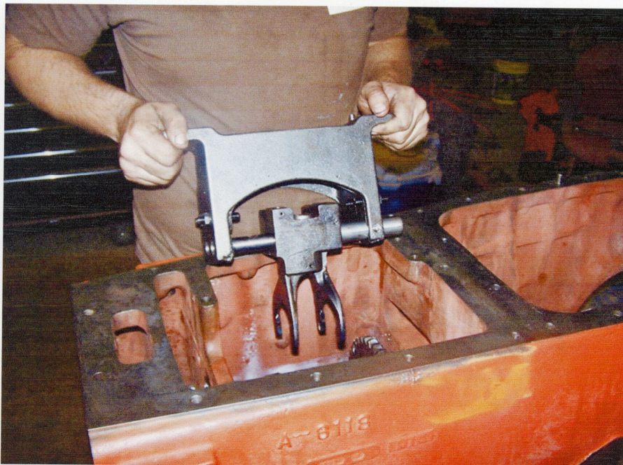
Reinstalling shifting forks
