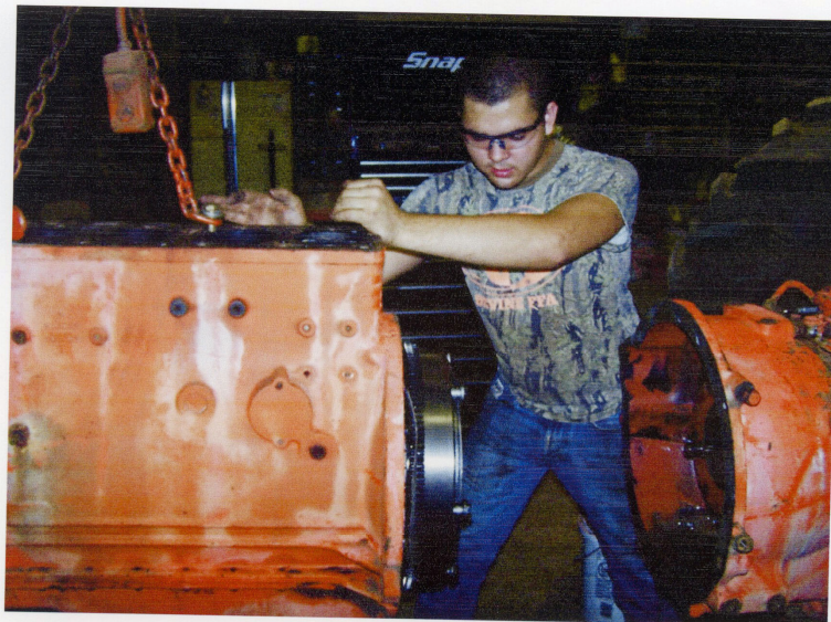
Removing engine from bell housing
