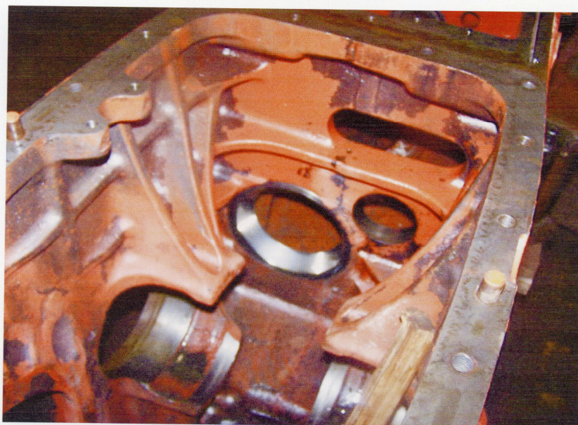
Empty transmission and rear end case
