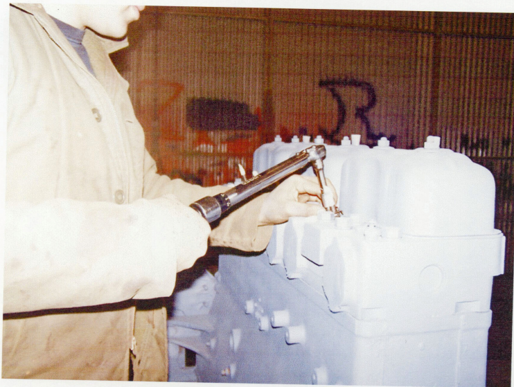
Torquing injector hold-downs
