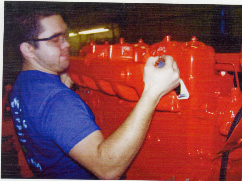
Installing intake manifold
