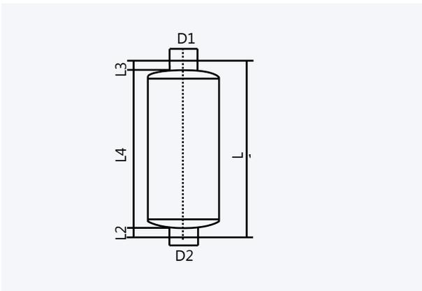
Silencer Schliro vertical with sleeve connection
