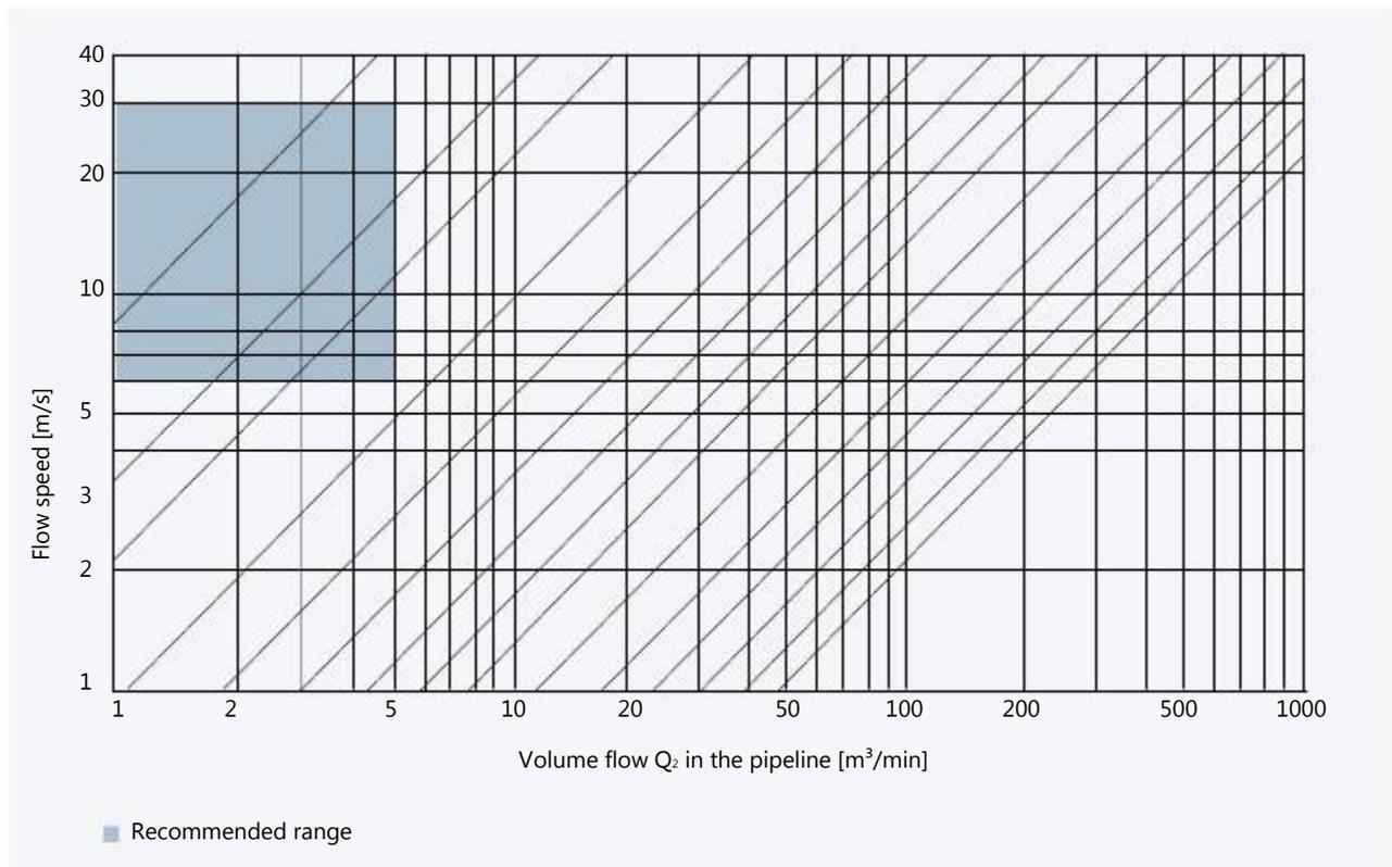
Volume speed  $c_2$  in the pressure pipeline
