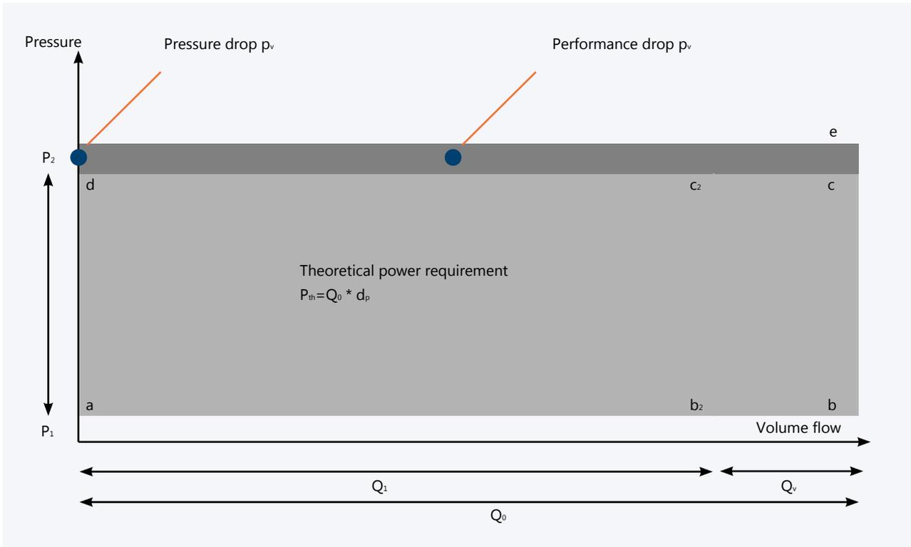
The pressure at outlet «pressure»  $p_2$  corresponds to the pressure at the blower inlet  $p_1$ .
