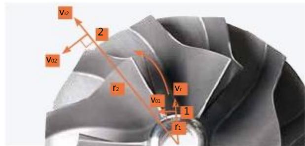
$$\text{Torque} = \dot{m}(r_2 v_{02} - r_1 v_{01})$$
