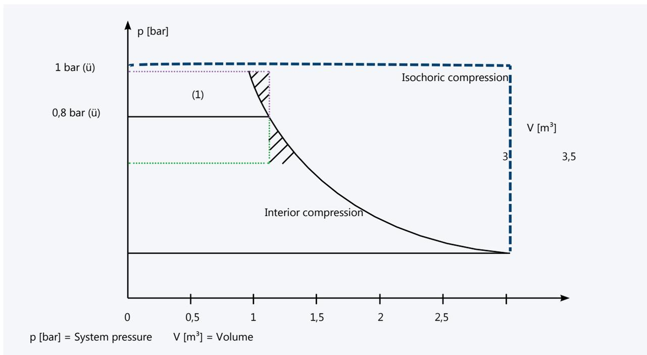
We can illustrate this power saving using the p-V diagram shown above. Assuming that the area of the diagram corresponds to the required power consumption, isochoric compression (of a positive displacement blower) for a system pressure of 1 bar ( $\ddot{u}$ ) would require the power as shown by the area bordered by the dashed line (-----). In this example, the stage compresses to 0.8 bar ( $\ddot{u}$ ) on the inside. This internal compression requires less power, as the solid line curve in the
