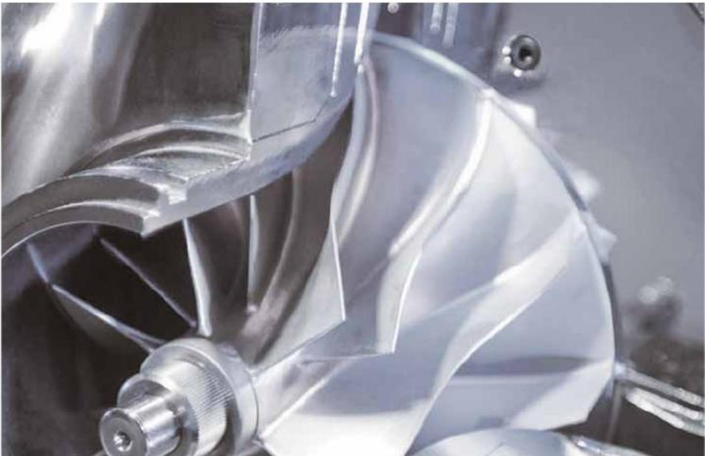
Even then, the blower stage based on the principle of a radial compressor was identical with today's modern turbo blowers. However, over time, the size and drive technology have changed significantly. Due to these developments, today's speed-regulated units are significantly more compact, more efficient and almost maintenance-free.
