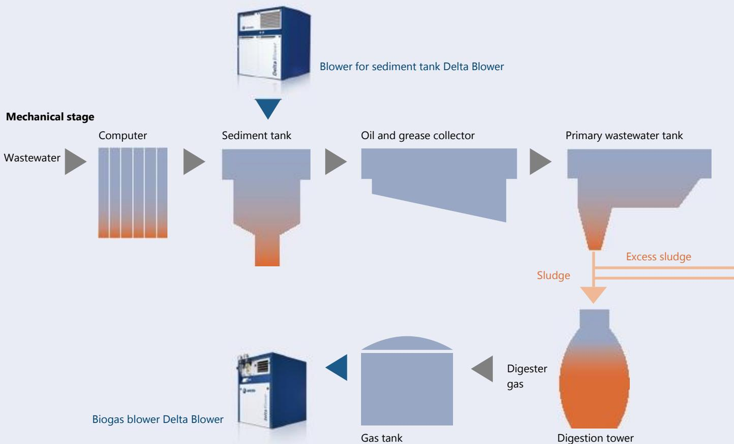
It is used sustainably to create energy to relieve the environment and remedy resource deficits. Due to the pressure increase of biogas blowers, the gas is transported to CHPs or generators where the converted energy can be used to heat buildings or greenhouses, for example. The produced gas is measured by AERZEN rotary piston gas meters. During sludge drying processes, AERZEN positive displacement blowers can be used for the
