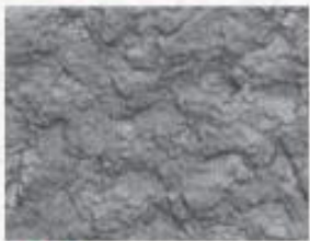
CSP 7 (heavy shotblast)
