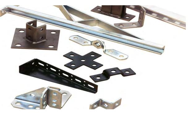
This section offers a full selection of fittings and accessories to complete our strut system. Fittings are made from hot rolled, pickled and oiled plate or strip steel in accordance with ASTM A1018 33,000 PSI min. yield, unless noted.
