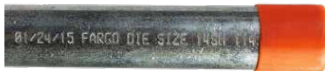
Above: close up of marking on Fargo splice requiring 14SH die index.
