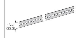
CLEATS: To reinforce load-bearing joints, cleats can be field made by cutting 21/4" (57.1) long segments from the widest slotted angle available.
