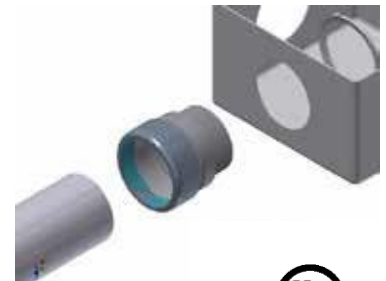
Unthreaded GRC/IMC/ EMT/PVC to Metal Box
