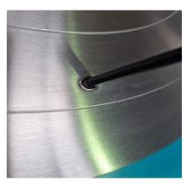
• Replace Bat Pins with blanking plugs using a 4mm Allen Key.
