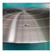
Blanking plugs sit just below flush with the wheelhead.
