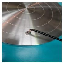
Remove Bat Pins using a 6mm Allen Key.
