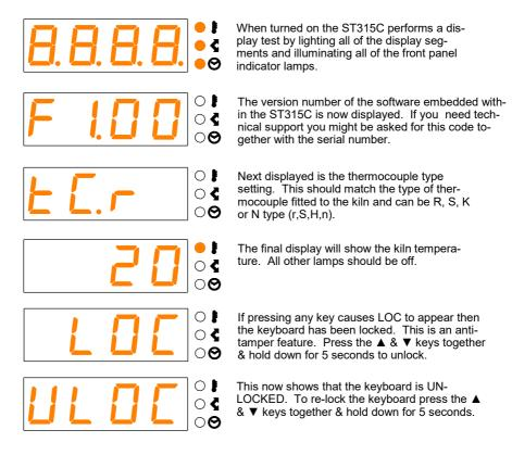
If any mimic panel lamps are on then the ST315C is firing. To stop the firing press the ightharpoonup key.
