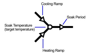
An ST315C firing segment comprises a ramp followed by a soak period. Two segments can be used for simple firing (biscuit firing for example) or several segments can be used per program for complex firing (crystal glazing or glass-making for example).
