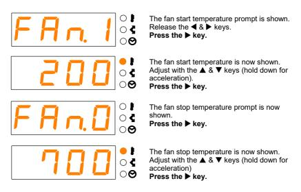
The ST315C will now reset and the new fan control temperatures will be stored.
