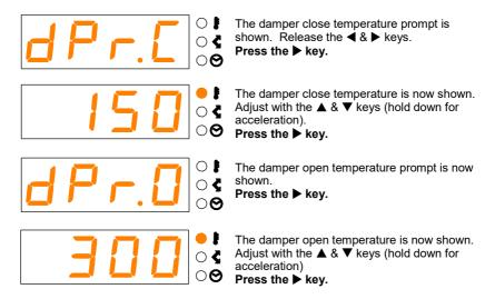
The ST315C will now reset and the new damper control temperatures will be stored.
