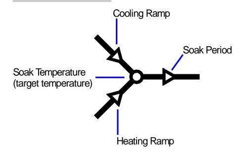
A CeraControl firing segment comprises a ramp followed by a soak period. Two segments can be used for simple firing (biscuit firing for example) or several segments can be used per program for complex firing (crystal glazing or glass-making for example).
