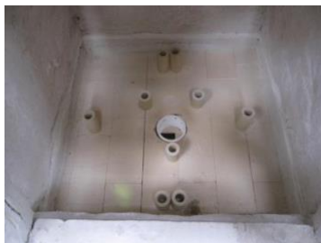
Props in place in kiln base
