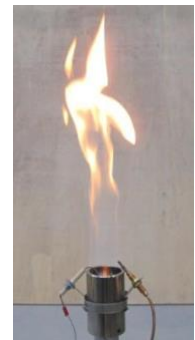
Yellow flame air intake valve closed
