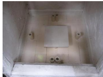
Bagwall in place above burner port
