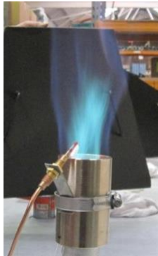
Blue flame air intake valve open
