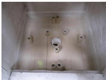
Props in place in kiln base
