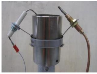
Burner, ignition, flame failure.
