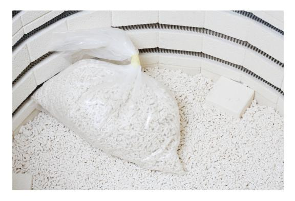
All new kilns will contain a bag of the Ultralite granular insulation. The loose-fill insulation in the kiln tends to settle during the kiln transportation. This bag of Ultralite material should be used to top up the granular insulation level, to just below the level of the support blocks. If the level is too high it may not allow the bottom kiln shelf to sit firmly on the support blocks.
