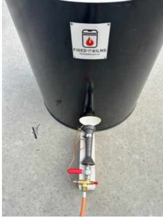
Above Image shows correct burner positioning
