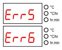
Error 5. Kiln temperature overshoot. The kiln temperature exceeds the desired temperature by at least 10°C / 20°C (installer selectable).
