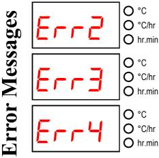
Error 2. Thermocouple or thermocouple wiring open circuit. Get thermocouple and wiring checked. Have thermocouple replaced if necessary.
