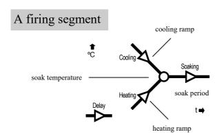
An ST315B firing segment comprises a ramp followed by a soak period. Two segments can be used for simple firing (biscuit firing for example) or up to 9 segments can be used per program for complex firing (crystal glazing or glass-making for example).
