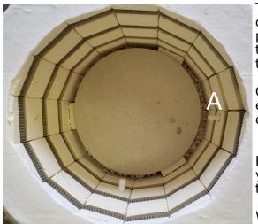
The kiln is provided with furniture applicable to the size of the firing chamber, we recommend the furniture is placed first on the base props bricks protruding through the Loosefill insulation, then 3 props are positioned equal distance apart across the kiln.
