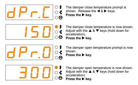
The ST215C will now reset and the new damper control temperatures will be stored.
