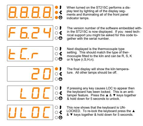
If any mimic panel lamps are on then the ST215C is firing. To stop the firing press the ▶■ key.
