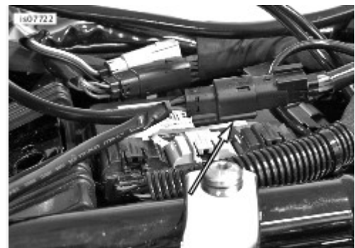
Figure 8. Rear Speaker Jumper Harness Routing
