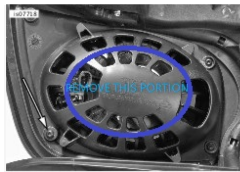
Figure 4. Speaker Grille Screws & Basket Cut Area
