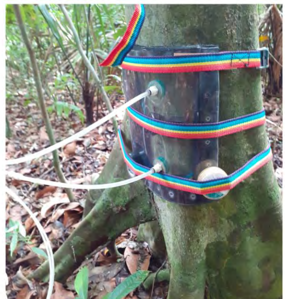
Extended Data Fig. 1 | Photograph of a typical tree woody surface flux measurement chamber. Each chamber has an inlet and an outlet that join to a laser methane analyser. See methods. For a fuller description of the method see Siegenthaler et al. 22 . Photograph by Josep Barba.
