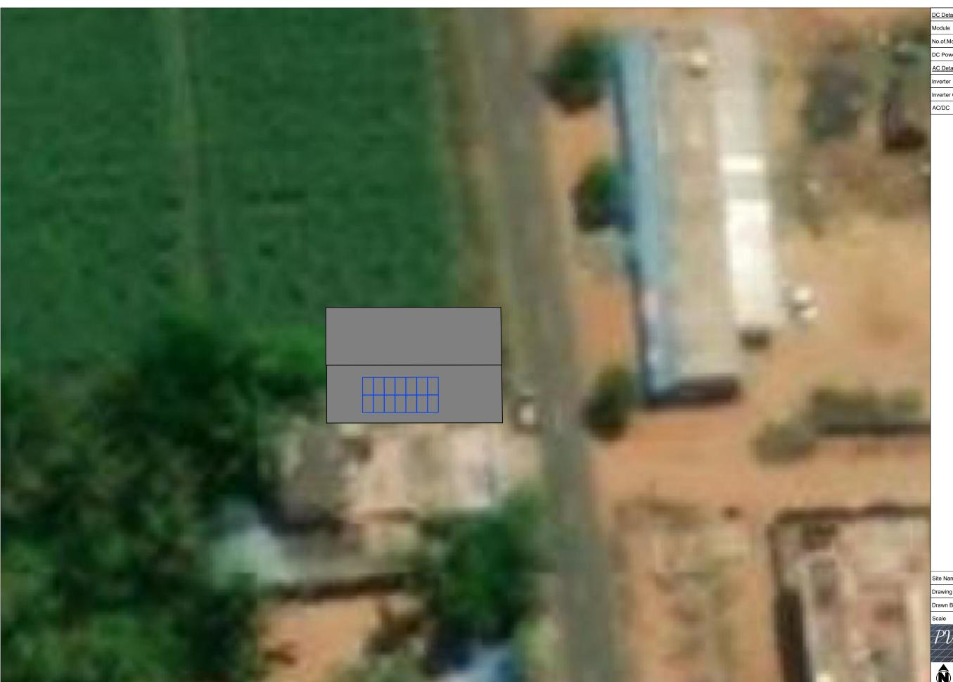
DC Details Module : TS250 (Tata Solar Power) - 250W No.of.Modules DC Power : 3.5kW AC Details : Fronius IG Plus 3.0-1 (240V) - 3kW nverter Inverter Quantity : 1
