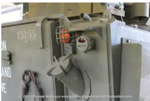
Above: Rear of M113MRV showing revised fixtures to right hand side of door. Tow bracket & chain is also carried by this vehicle.
