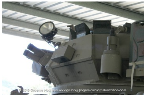
Above: Standard turret detail including smoke dispensers and spotlight.
