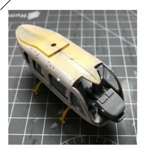
Remember to fit the glazing before joining the fuselage together. Use Kristal Klear or similar to fix and then leave for a few hours to set.
