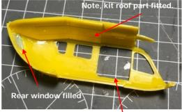
Doorway cut out Note\* The Heller kit has both doors separate and are in clear plastic.
