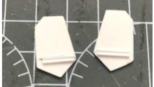
New plasticard tailplane fins with new plastic channel locating strips
