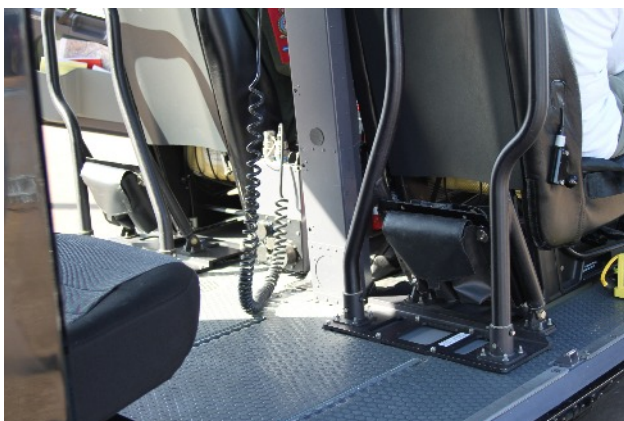
Above: View forward from the rear cabin seats showing fixing of the grab bars.
