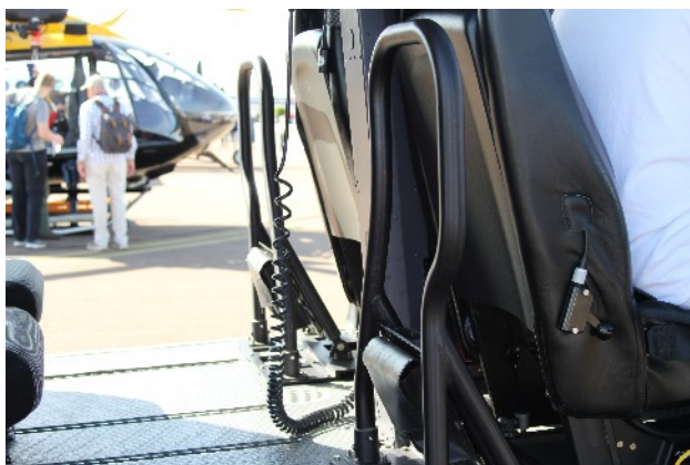
Above: Front cabin seats are black with light grey cushions. Note* two bars behind seats which will need to be made From sprue, wire or plastic rod. These fit into the strip behind The front seats.
