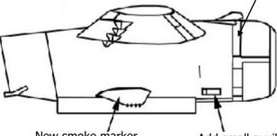
New smoke marker Ejector unit. Part No 20 Starboard side outer Engine only. Add small auxiliary intake cover to both outer engine cowlings Part Nos 27 and 28
