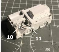
Lastly, fit steering Wheel Part 10 & Safety bar Part 11. Note: I replaced the Steering column With thin Brass Rod for strength.
