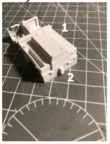
Fit Part 2 to the rear of Part 1 (Main body) This will need a small amount of sanding for a perfect fit.
