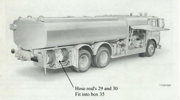
TRUCK, FUEL SERVICING, Aircraft, 10 ton, 6 x 4, 3,000 Gal, D/P, AEC Mammoth Major TG 6 RB (Mk 1 fitted with 'Streamline' filters)
