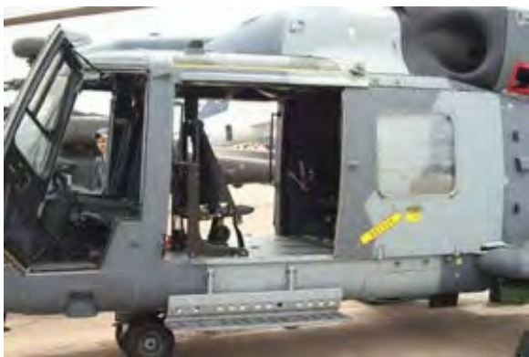
Left: Detail of the cabin door, cockpit door and step.
