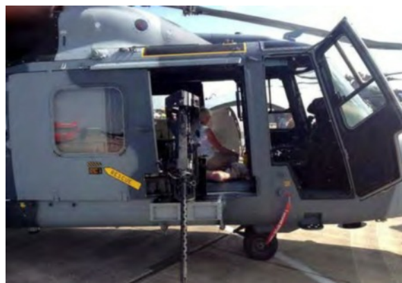
Left: Machine gun and mount detail. The gun can be mounted either side of the cabin.
