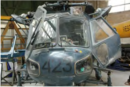
Nose improvement bits Including aerials, round cap & thin bar across nose. This also shows the position of the floatation buoys on the floats.
