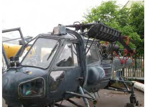
Good general details including nose and side. Note the gun sight in the roof.
