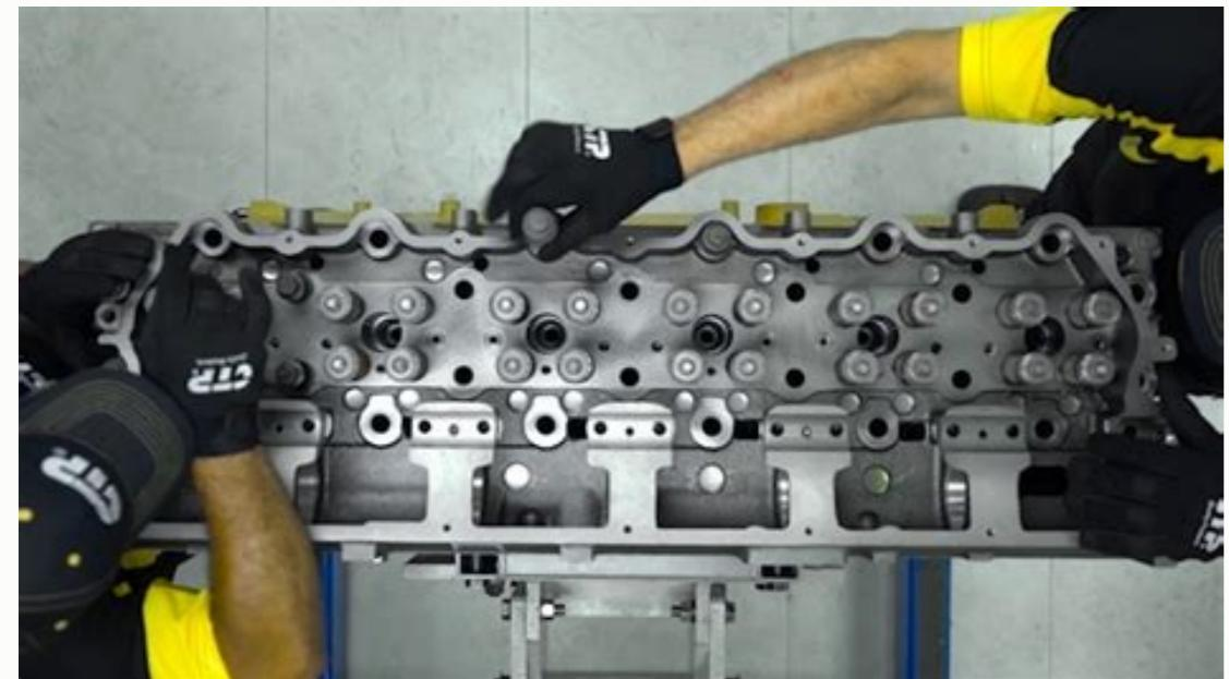
2. Check the screw holes carefully, otherwise the thread of the cylinder block has no damage. 3. Install a new head gasket (3). Note: Use the correct size control screws in the cylinder head to avoid damaging the head gasket. 4. Apply the head with a suitable lifting device. Place the cylinder head block on the cylinder block pins.
