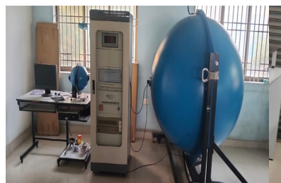
LED lamp and LED chip LM79 testing testing integrating sphere
