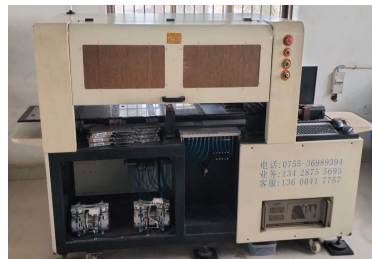
Fully automatic SMT LED mounter 20K pcs per hour mounting speed with 4 head camera
