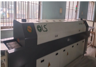
SMT reflow welding machine with 8+8 zone
