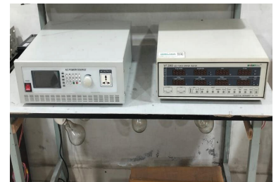
LED driver testing equipments, Variable AC source and THD, Efficiency, PF tester
