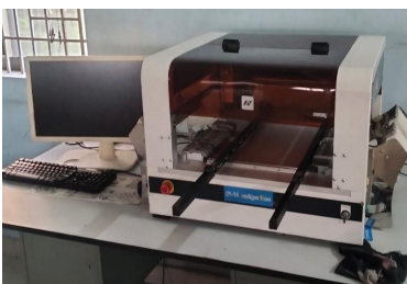
SMT pick and place machine for LED driver Assembly
