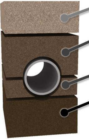
4. Residual backfill
