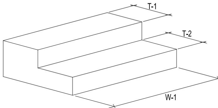
**4.5.4.6 Stair Risers** Stair risers shall have a minimum uniform height of 6 inches (15.2 cm) and a maximum height of 12 inches (30.5 cm), with a tolerance of ½ inches (12.7 mm) between adjacent risers.
