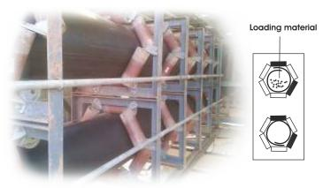
Each new installation of pipe conveyors is unique and presents special design requirements. In order to ensure the compatibility of the belt with the conveyor, the Oriental Technical Team is proactive in carrying out design discussions with the OEMs, which are followed by simulation, prototyping and testing on our live rigs specially designed for this purpose by us.
