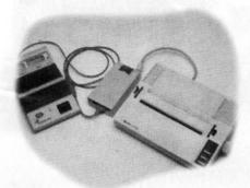
Printout option is available along with an EVM by using a Download Adaptor Unit (DAU). With the help of a modem, the DAU can also enable transmission of voting information to a distant centralized computer.
