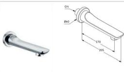
KLUDI BALANCE BATH FILLER bath filler DN 20 wall fastening projection 170 mm flow class C s-pointer aerator M 24 x 1C separate connector G 3/4 for pre-installation
