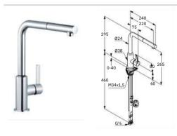
KLUDI L-INE S single lever sink mixer DN 15 solid lever single hole mounted ceramic cartridge flow regulator M 16 x 1 flow rate 8,2 l/min at 3 bar swivelling (360°) pull-out spout protected against back flow flexible hoses G 3/8 with shank fastening
