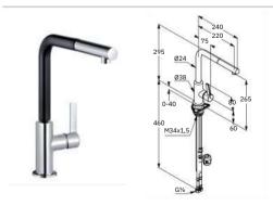
KLUDI L-INE S BLACK RETRACTABLE single lever sink mixer DN 15 solid lever single hole mounted ceramic cartridge flow regulator M 16 x 1 flow rate 8,2 l/min at 3 bar swivelling (360°) pull-out spout protected against back flow flexible hoses G 3/8 with shank fastening
