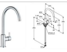
KLUDI BINGO STAR XS single lever sink mixer DN 15 solid lever single hole mounted flow rate 7,6 l/min at 3 bar PCA caché-Laminar-flow regulator M 16,5 x 1 ceramic cartridge swivelling spout (360°) rapid installation set flexible hoses G 3/8
