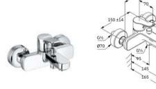
KLUDI PURE&EASY BATH SHOWER MIXER single lever bath- and shower mixer DN 15 wall fastening solid lever ceramic cartridge with hot water limitation flow regulator M 24 x 1 flow class C/B autom. diverter shower/bathtub shower outlet G 1/2 protected against back flow s-connections
