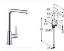
KLUDI L-INE S single lever sink mixer DN 15 solid lever single hole mounted ceramic cartridge Laminar-flow regulator M 18 x 1 flow rate 7,1 l/min at 3 bar swivelling spout (360°) flexible hoses G 3/8 with shank fastening
