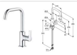
KLUDI PURE&EASY 200MM BASIN MIXER single lever basin mixer DN 15 single hole mounted solid lever ceramic cartridge PCA aerator M 18 x 1 flow rate 5 l/min at 3 bar swivelling spout without pop-up waste flexible hoses G 3/8 rapid installation set
