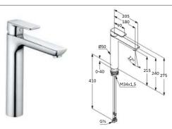
KLUDI PURE&STYLE 215MM BASIN MIXER single lever washbowl mixer DN 15 single hole mounted solid lever ceramic cartridge with hot water limitation flow regulator M 24 x 1 flow rate 7 l/min at 3 bar without pop-up waste flexible hoses G 3/8 rapid installation set spout height lower edge 215 mm
