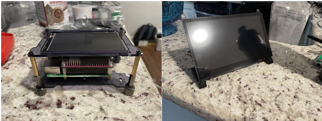
Figure 8. A 5” and 7” screen prototype for low-cost gaming devices that also run full nodes. Each were constructed with Raspberry Pi 4B in a modular manner to make replacement/repair inexpensive.
