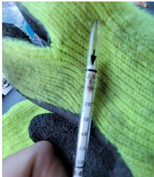
Additional monitoring of H 2 S 5 months post treatment 11/18/22 still undetectable H 2 S.
