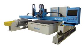
The AKS "dura-kut" is also available in the "dura-max" model which is an extra heavy-duty version specifically designed for wider width bridge beams and heavier loads for multiple torches and multiple carriages. The AKS "dura-max" comes in widths of 16', 18', 20', 22' and 24' and offers multiple plasma torches, both straight and AKS "robo-kut" 5-axis Bevel Head, and multiple oxy-fuel torch(es) technology.
