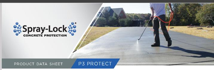
**P3 Protect** is a spray-applied product, based on Spray-Lock Concrete Protection (SCP) colloidal silica technology, which provides a permanent improvement that increases the durability and life cycle of Portland cement concrete.
