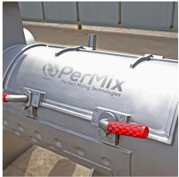
Access Door of PTS Plow Mixer
