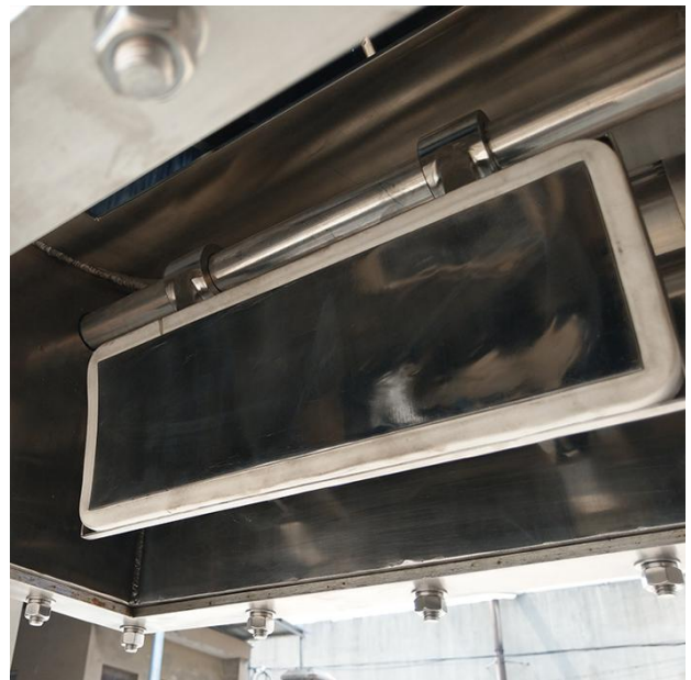
Internal View of Discharging Housing
