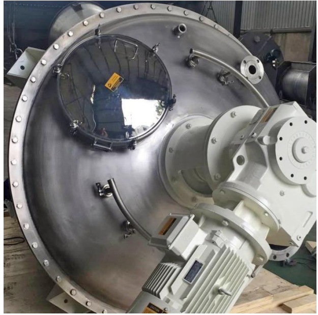
Manway and Liquid Adding Nozzles
