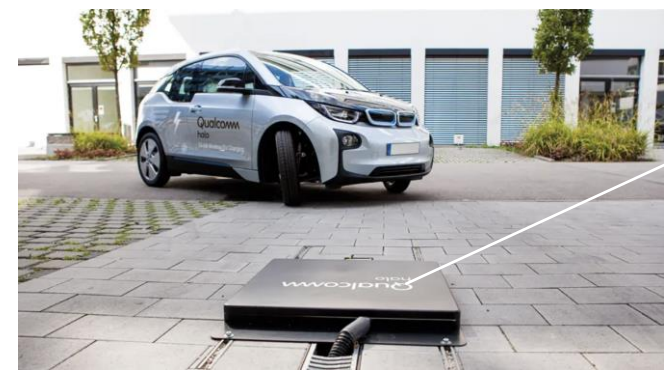
Wireless induction pad over concrete
