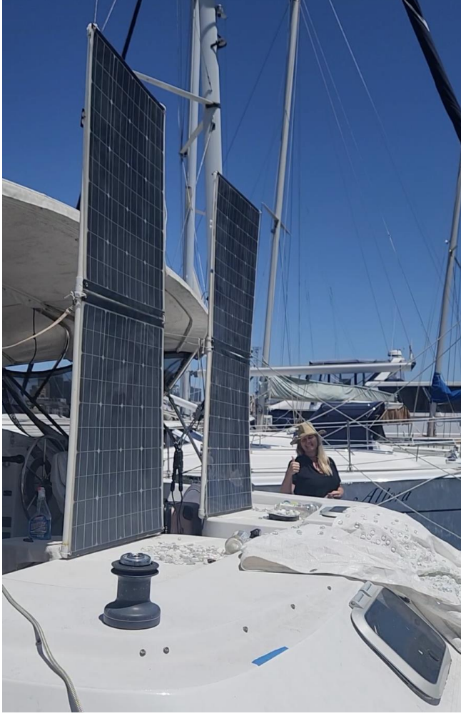
White composite, glass 53 watts, 24% increase
