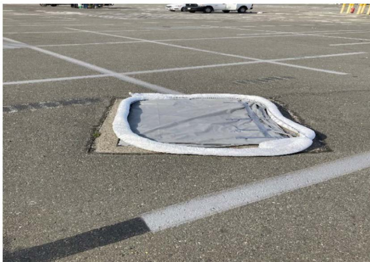
Caption: Storm drain sampling- Space X69/121, 8/14/2023, Port of Oakland.
