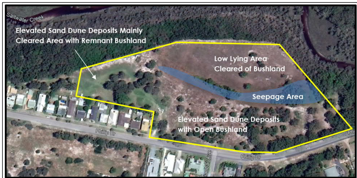
Figure 17: The site's geotechnical setting (RGS, 2022).
